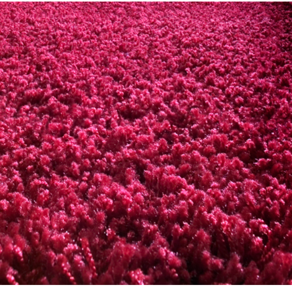
Carpet made with spun yarn — many small pieces of yarn are woven together into long strands
